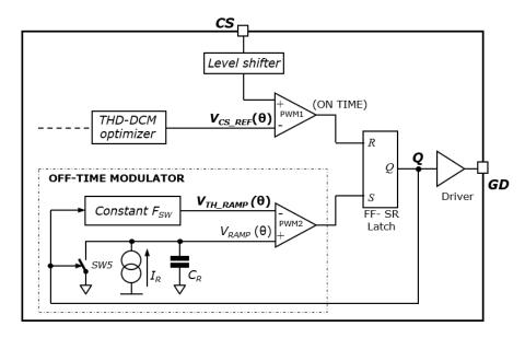
Figure 7. OFF-time modulator - details
