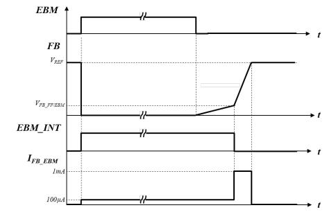
Figure 13. External Burst-Mode (EBM) function - timing
