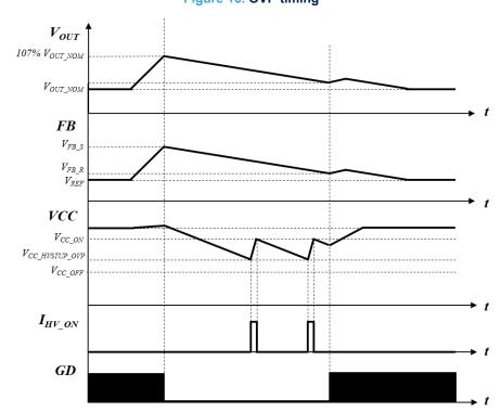
Figure 16. OVP timing
