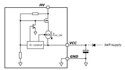
Figure 10. Embedded high voltage start-up circuitry
