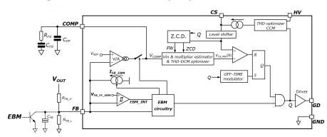
Figure 12. External Burst-Mode (EBM) function - circuit details
