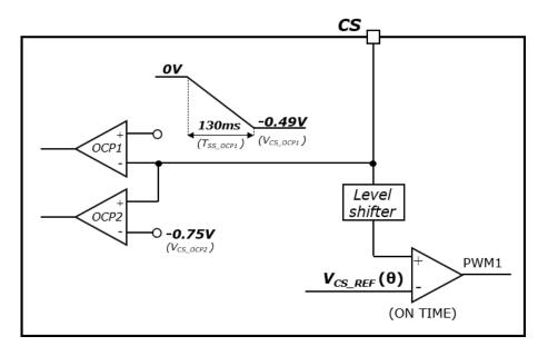
Figure 11. Soft-start circuitry details
