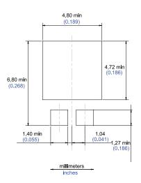
Note: For package and tape orientation, reel and inner box dimensions and tape outline please check TN1173
