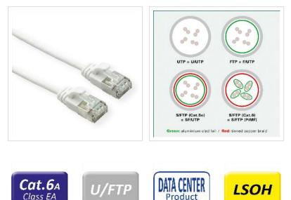
Category 6a twisted-pair patch cable with shielded RJ-45 connectors on both sides. Particularly thin and flexible cable with individual pairs of wires in aluminium-laminated foil for use in confined spaces, such as in data centres.
