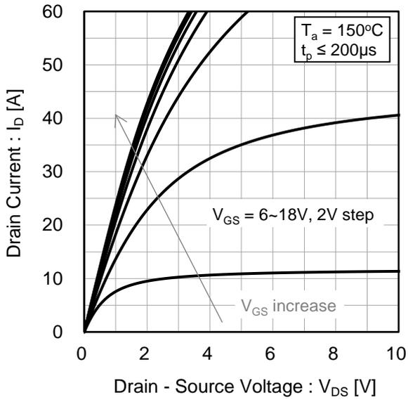
Fig.8  $T_a = 150^\circ\text{C}$  Typical Output Characteristics(II)
