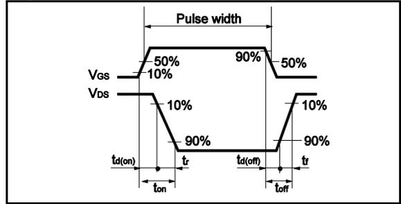
Fig.2-3 Waveforms for Switching Energy Loss
