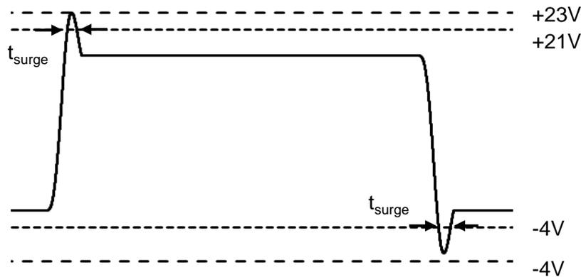
\*6 Please be advised not to use SiC-MOSFETs with  $V_{GS}$  below 10V as doing so may cause thermal runaway.
