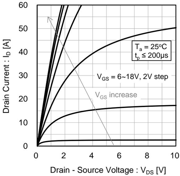
Fig.5  $T_a = 25^\circ\text{C}$  Typical Output Characteristics(II)
