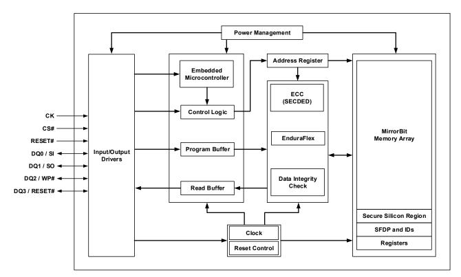
Figure 2. Logic Block Diagram Monolithic Device
