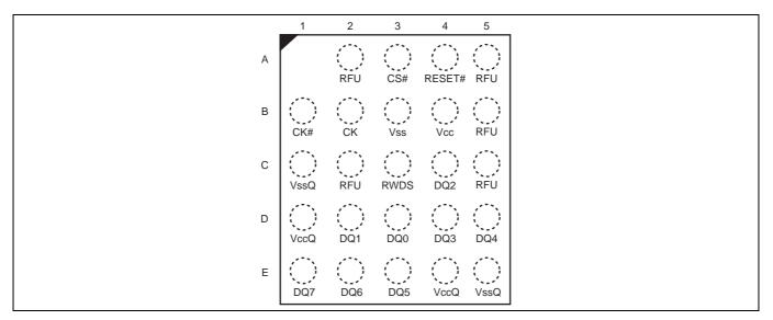
Figure 3324-ball FBGA, 6 × 8 mm, 5 × 5 ball footprint, top view
