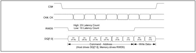
Figure 11 Register write operation<sup>[39, 40]</sup>
