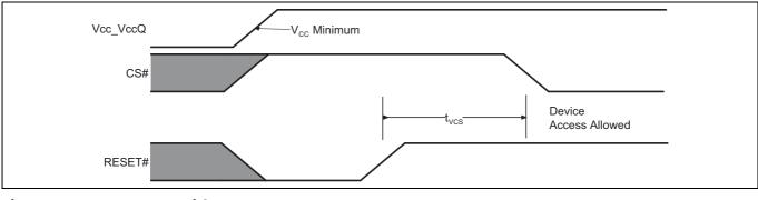
Figure 20 Power-up with RESET# LOW
