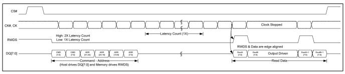
Figure 12 Active clock stop during read transaction (DDR)<sup>[46]</sup>
