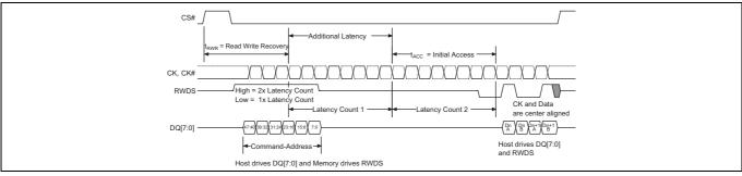
The clock is not required to be free-running. The clock may remain idle while CS# is HIGH.
