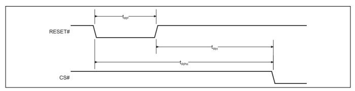
Figure 22 Hardware reset timing diagram
