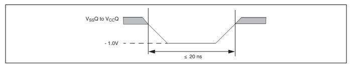
Figure 17 Maximum negative overshoot waveform
