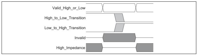
Figure 23 Key to switching waveforms
