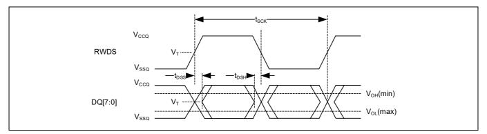
Figure 32 DDR output timing reference levels
