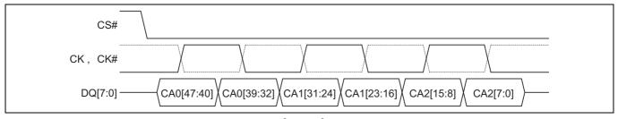
Figure 6 Command-address (CA) sequence<sup>[6, 7, 8, 9]</sup>
