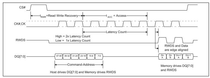
Figure 1 Read transaction, initial latency count<sup>[1]</sup>
