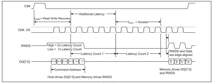
Figure 9 Read transaction with initial latency<sup>[23-31]</sup>
