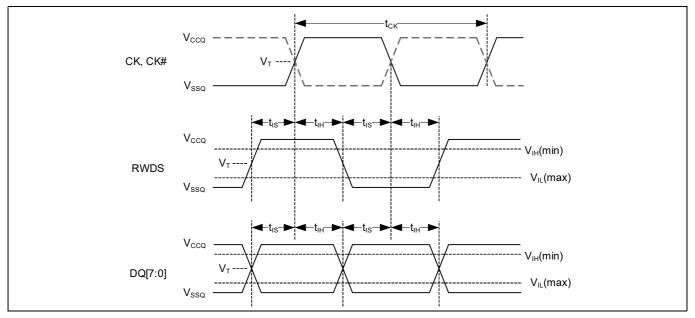
Figure 31 DDR input timing reference levels
