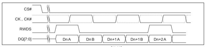
Figure 8 Data placement during a write transaction<sup>[19-22]</sup>
