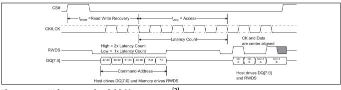
Figure 3 Write transaction, initial latency count<sup>[2]</sup>
