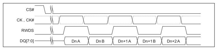
Figure 7 Data placement during a read transaction<sup>[14-18]</sup>
