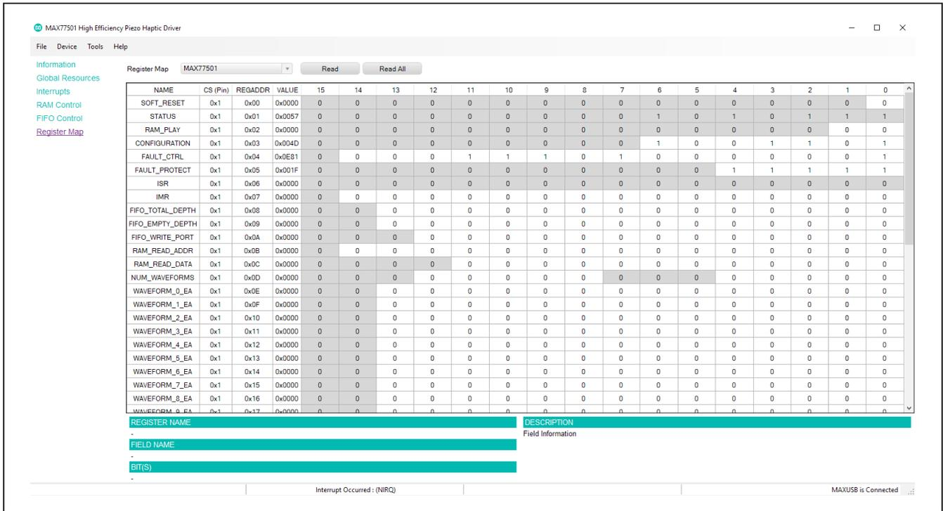
Figure 11. EV kit GUI Register Map Tab
