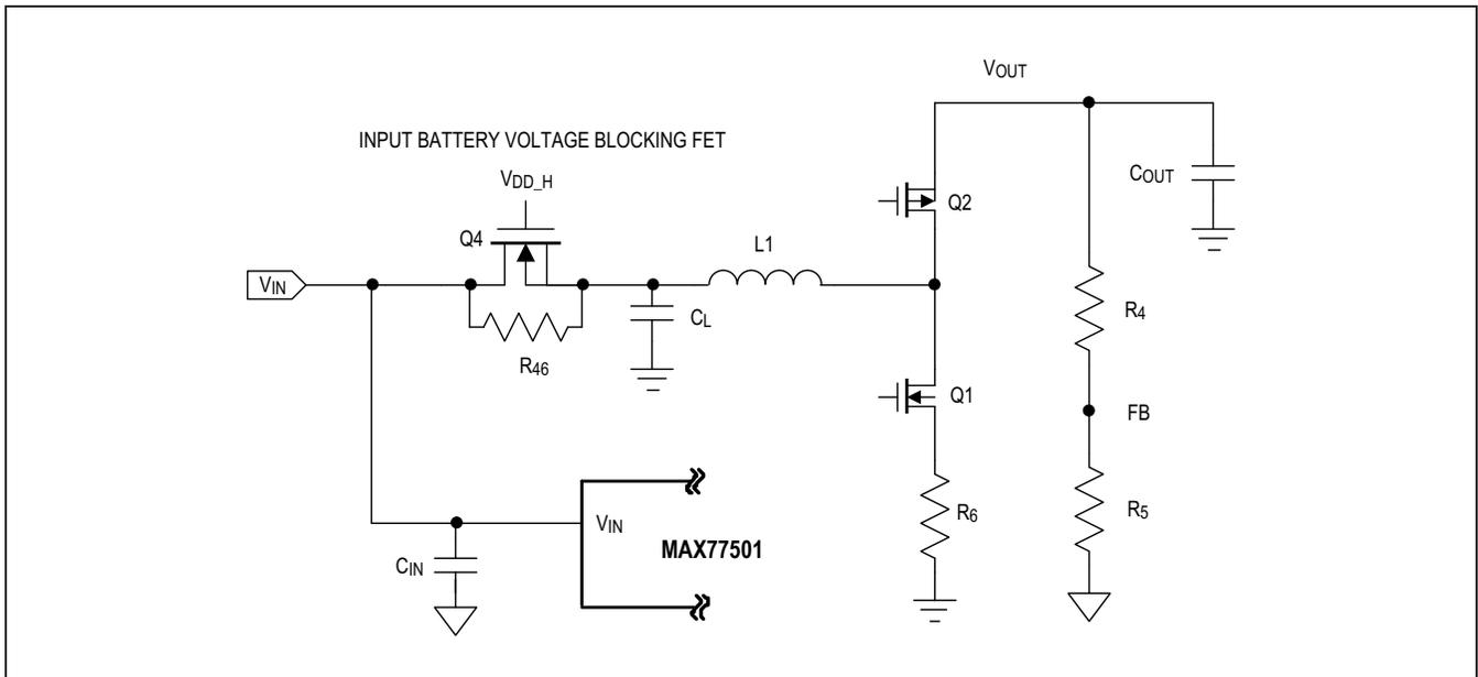
Figure 4. Input Battery Voltage Blocking Diagram
