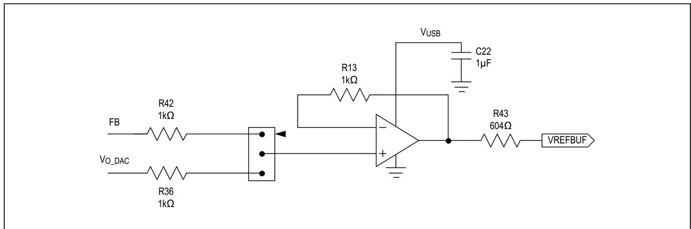
Figure 3. VREFBUF Feedback and DAC Measurement Amplifier Diagram
