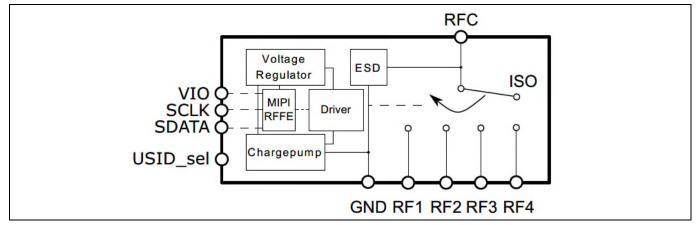
Figure 1 BGSA14M2N10 Block diagram
