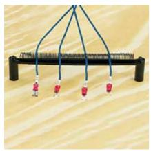
System consists of harness board springs and spring holders to hold wire ends taut. When harness is removed from board wires simply pull out from spring. Each SHH Spring Holder is supplied with (1) rigid wire piece to hold the spring laterally and two #8 (M4), 2.0" (50.8) hex head wood screws. Two sizes of spring holders are available for use with PBSC1 and PBSC6 springs.
