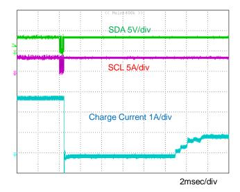
Figure 17. Charge Current Setting Change (3.072A to 1.024A)
