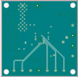
Figure 29. Middle 1 Copper Trace Layer (Ground)
