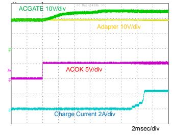
Figure 3. Adapter Insert to ACOK
