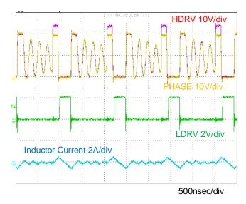
Figure 7. Fixed Frequency Mode Light Load Switching Waveform
