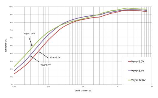
Fig.24 SLLM Mode Output Current vs. Efficiency
