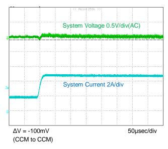
Figure 11. No-Battery System Current Load Transient (2A to 5A)
