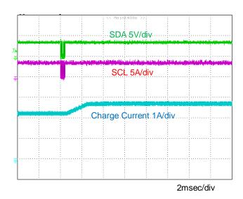
Figure 14. Charge Current Setting Change (2.560A to 3.072A)
