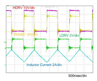
Figure 8. Continuous Conduction Mode Switching Waveform
