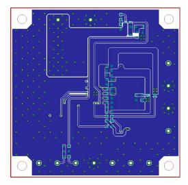
Figure 31. Bottom Copper Trace Layer (Signal and Ground)
