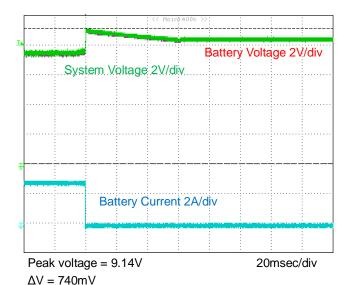
Figure 18. Battery Removed
