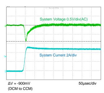
Figure 10. No-Battery System Current Load Transient (0A to 5A)
