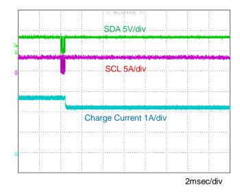
Figure 15. Charge Current Setting Change (3.072A to 2.560A)
