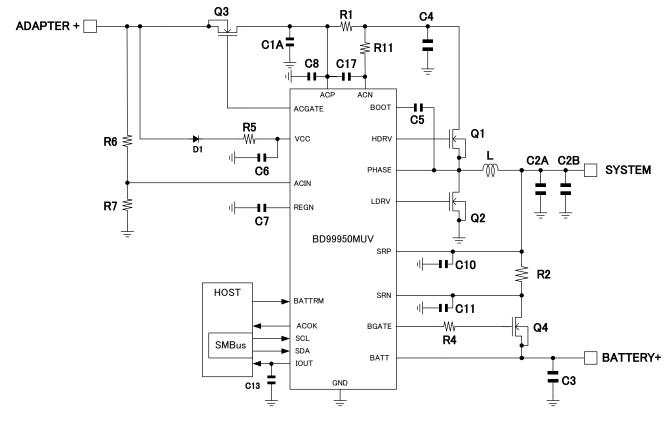
Figure 34. Example of Application Circuit (Minimum Component Configuration)
