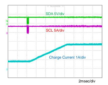
Figure 16. Charge Current Setting Change (1.024A to 3.072A)
