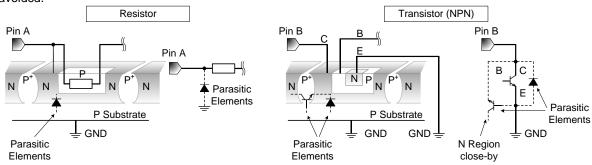
Figure 36. Example of monolithic IC structure
