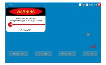
VFL contains four status modes: Steady mode", "Evasive 1Hz", "Evasive 2Hz" and "Time off". Click button "Steady mode" to enter steady status; click button "Evasive 1Hz" and "Evasive 2Hz" to enter pulse mode; click button "Time off" and VFL is turned off for selected time intervals: may select (5 mins, 10 mins, 30 mins, 60 mins and 120 mins).
