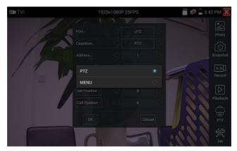
Enter address of PTZ camera; after finishing the parameter settings, you can press the key enter or click the icon to call the dome camera menu.
