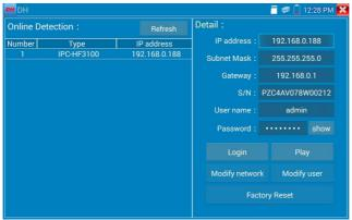
From the Pop up stream menu, select mainstream or secondary substream to test.
