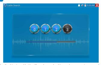
Use the blue Combination cable identifier and network cable tester's copper pointer to touch all the cables in the bundle when searching for the other end of the cable. The cable that gives off the loudest tone is the cable connected to the tester. Press the + or - buttons on your blue cable identifier to adjust the volume
