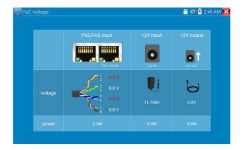
Connect a network cable from a PoE switch to the IP tester's PSE IN port. Connect an IP camera or other PoE device to IP tester's LAN port. The PoE voltage and the cable's pin connection status show on the screen.
