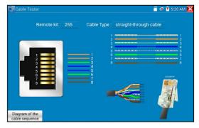
Test LAN cable or telephone cable.
