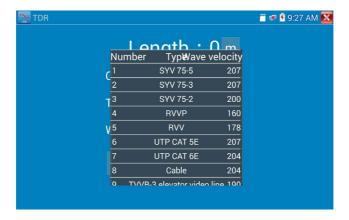
**User-defined calibration**: Choose the cable 100 meters to 200 meters (more than 50 meters); click "Cable" and "Type" to select user-defined 1 for calibration. Eleven groups can be set.
