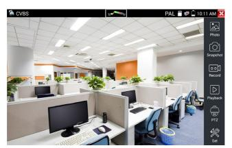
Select relative functions on the right side toolbar to operate functions including "Photos", "Snapshot", "Record", "Playback", "PTZ", and "Set".
