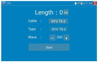
BNC cable, network cable, RVV control cable, Telephone line and TVVB cable etc. can be tested with the TDR cable tester. Eleven groups of user-defined cables can be saved. Click "Cable" and "Type" to select cable and tap "Start" to start testing. If selecting built in cable type for testing, click "+" and "-" to adjust the wave speed.
