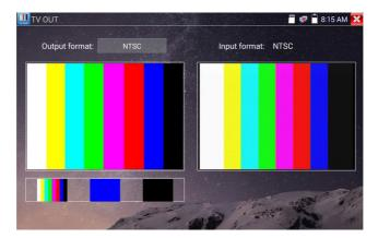
BNC loop test: Tester can send and receive color bar generator through the tester's "CVBS out" and "CVBS in" port for testing transmission channels, such as video balun, BNC video cables, etc. Connect the tester's "CVBS OUT" port to the balun transmitter's BNC input port and connect the tester's "CVBS IN" port to balun receiver's BNC output port. The same can be done with a single BNC cable.
