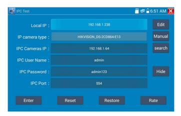
**Local IP**: This is the tester's IP address. Click "Edit" to enter "IP settings" and change the tester's IP address settings.
