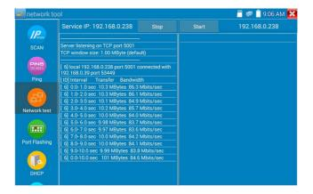
b). Start send packet test: Using the second IP tester, type in the Server's IP address at the top right corner of the screen. This app is used to send packets for network speed testing. Click the "Start" button to send the packets and start testing.
