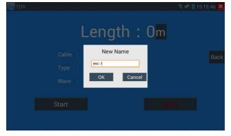
**Application:** TDR test is the use of the pulse reflection method to transmit pulse signals for testing cable. When cable is open or short circuit a reflected pulse is generated and the tester receives and processes the reflected wave and measurement results are displayed on the screen. TDR can test cable open circuit and short circuit and help engineer quickly find the cable's problem location.
