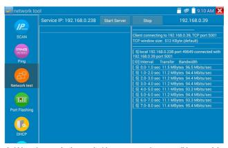
Network bandwidth testing can also be tested with a computer using compatible network bandwidth testing software. Install network bandwidth testing software on a computer, as a test Client or Server, to do the mutual testing with the tester. If using a computer as the server, the computer IP address is: 192.168.0.39
