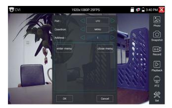
Enter address of PTZ camera; after finishing the parameter settings, you can press the key (ENTER) or
