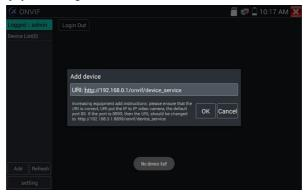
Click the button "Refresh", tester will scan the ONVIF camera again. Click the newly displayed ONVIF camera on the "Device List". The tester will show the IP camera's relative information and settings.
