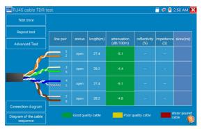
**Advanced Test:** tests cable pair status, length, attenuation, reflectivity, impedance, skew, and other parameters.
