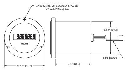
Panel cutout: 2.16" [54.9] Dia. Mounting holes: 0.125" [3.2] Dia. on 2.44" [62.0] B.C.
