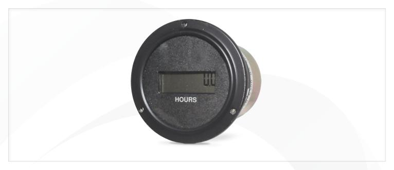
The Model 720 Electronic Hour Meter offers a large 8 digit LCD display, (9999999.9) 0.32" (8mm) high, with an input operating voltage of 85-500VAC. The front of the unit is totally sealed, and the Hour Meter is housed in a rugged steel enclosure that is interchangeable with the Redington Model 720 Electro Mechanical Hour Meters. The wide operating voltage makes this product ideal for almost any application.
