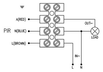
When all wires are connected locate the terminal block onto the two pins on the back plate.
