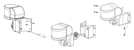
Feed the supply and load wires through the grommets in the sensor and pass through the cable clamp and connect as follows:
