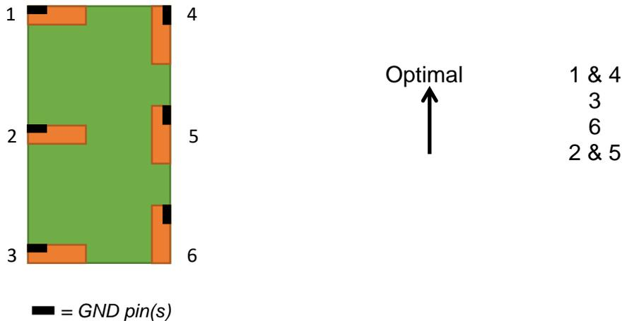
The antenna should be aligned with the PCB edge if possible, preferably with the GND pin(s) close to a corner.
