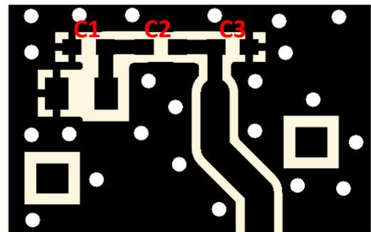
The antenna needs a matching circuit to adjust the resonant frequency balance. When delivered, the evaluation board is tuned for optimum balance at the 2.4 GHz band. The component values for this setup are:
