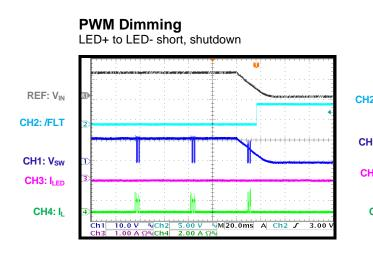
**PWM Dimming** LED+ to LED- short entry and recovery
