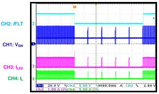
**PWM Dimming** One or more LED short faults, shutdown
