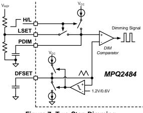
Figure 7: Two-Step Dimming
