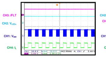
**PWM Dimming** LED+ to LED- short, start-up
