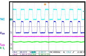
Buck-boost mode, 8 LEDs,  $V_{LED}$  = 24V,  $V_{IN}$  = 12V,  $f_{SW}$  = 410kHz, L = 10µH,  $T_A$  = 25°C, unless otherwise noted.
