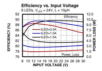
Buck-boost mode, 8 LEDs,  $V_{LED}$  = 24V,  $V_{IN}$  = 12V,  $f_{SW}$  = 410kHz, L = 10µH,  $T_A$  = 25°C, unless otherwise noted.
