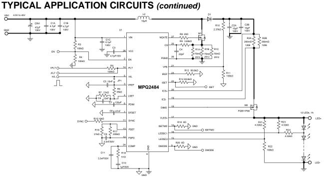
Figure 17: Typical Application Circuit for Boost Topology (Two-Step Dimming)
