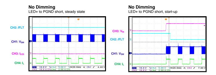
Buck-boost mode, 8 LEDs,  $V_{LED}$  = 24V,  $V_{IN}$  = 12V,  $f_{SW}$  = 410kHz, L = 10µH,  $T_A$  = 25°C, unless otherwise noted.
