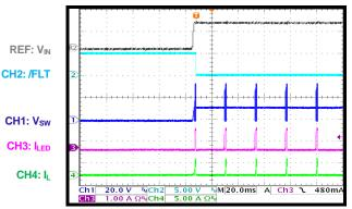
No Dimming One or more LED short fault, steady state CH2: /FLT CH1: Vsw CH3: ILED
