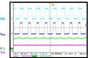
Boost mode, 12 LEDs,  $V_{\text{LED}}$  = 36V,  $V_{\text{IN}}$  = 12V,  $f_{\text{SW}}$  = 410kHz, L = 10µH,  $T_{\text{A}}$  = 25°C, unless otherwise noted.
