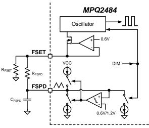
Figure 8: Frequency Spread Spectrum
