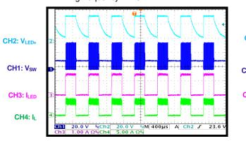
Two-Step Dimming Start-up through VIN
