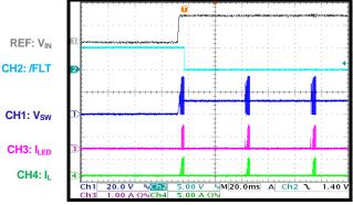
Two-Step Dimming One or more LED short faults, shutdown
