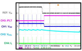
**Two-Step Dimming** LED open fault entry
