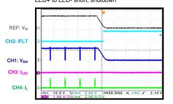
Two-Step Dimming LED+ to LED- short entry and recovery
