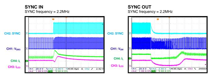
**PWM Dimming Steady State**
