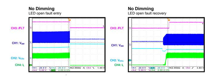
Boost mode, 12 LEDs,  $V_{LED}$  = 36V,  $V_{IN}$  = 12V,  $f_{SW}$  = 410kHz, L = 10µH,  $T_A$  = 25°C, unless otherwise noted.
