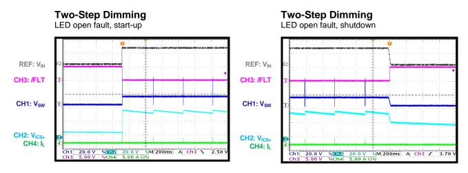
Two-Step Dimming LED open fault entry
