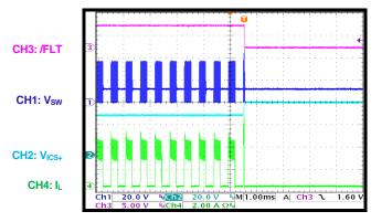
**Two-Step Dimming** LED open fault recovery
