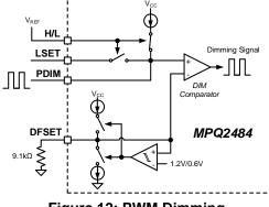
Figure 12: PWM Dimming
