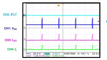
**PWM Dimming** One or more LED short faults, start-up
