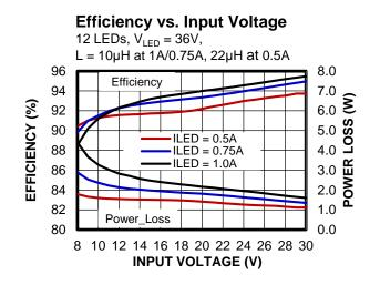
Boost mode, 12 LEDs,  $V_{LED}$  = 36V,  $V_{IN}$  = 12V,  $f_{SW}$  = 410kHz, L = 10µH,  $T_A$  = 25°C, unless otherwise noted.
