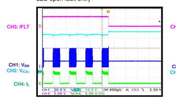
Two-Step Dimming LED open fault recovery
