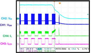
Boost mode, 12 LEDs,  $V_{LED}$  = 36V,  $V_{IN}$  = 12V,  $f_{SW}$  = 410kHz, L = 10µH,  $T_A$  = 25°C, unless otherwise noted.
