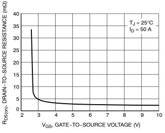
Figure 3. On-Resistance vs. Gate-to-Source Voltage
