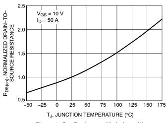
Figure 5. On-Resistance Variation with **Temperature**
