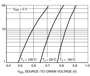
Figure 10. Diode Forward Voltage vs. Current
