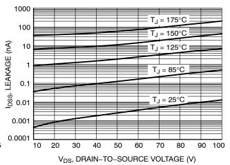
Figure 6. Drain-to-Source Leakage Current vs. Voltage
