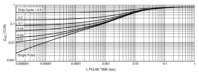
Figure 13. Transient Thermal Impedance
