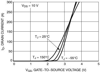
Figure 2. Transfer Characteristics
