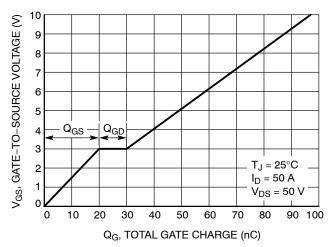
Figure 8. Gate-to-Source Voltage vs. Total Charge
