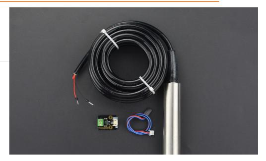
technology. The level transmitter receives different pressures at different depths of liquid, which can be converted into corresponding current signals and output through the sensor. In this way, the depth of liquid can be measured.
