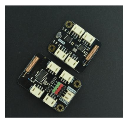
receiver has a corresponding pairing function to ensure that only the paired transmitting device can control the receiver, the receiver supports four working modes: inching, latching, self-locking, and interlocking. It can be paired with EV1527 coded transmitters. One receiver can be paired with up to 32 transmitters. The
