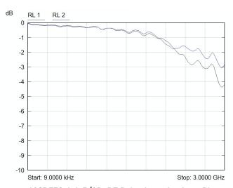
109RF50-1-A-5/2D RF Relay Insertion Loss Plots
