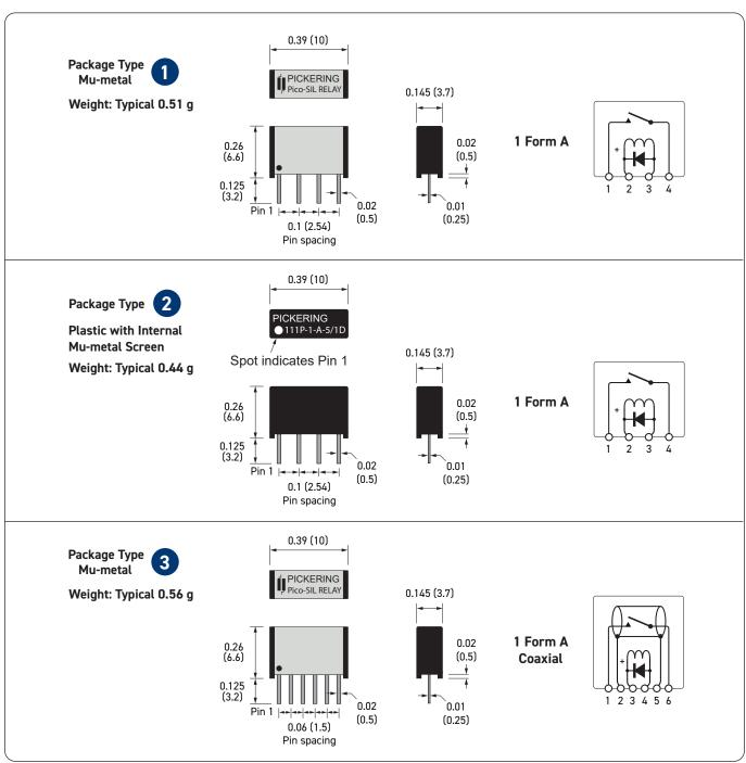
Pin Configuration, Weights and Dimensional Data (dimensions in inches, millimeters in brackets)
