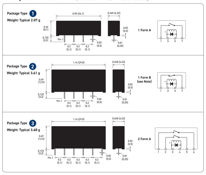
**Important:** Where the optional internal diode is fitted or for all Form B types, the correct coil polarity must be observed, as shown by the + symbol on the schematics.
