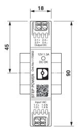
Figure 6 Device dimensions (dimensions in mm)
