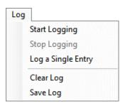
Click **Start Logging** to start the logging function. Each time the program polls the ALS information from the device, it will create a new log entry showing the raw data values, the calculated lux value, the values of various control registers, and the values entered by the user into the text fields near the bottom right corner of the window.
