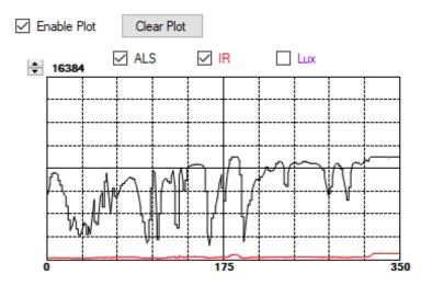
The scale of the Y-axis of the plot can be adjusted by clicking on the small up and down arrows at the top left corner of the plot. The scale can be set to any power of 2 from 64 through 65536.
