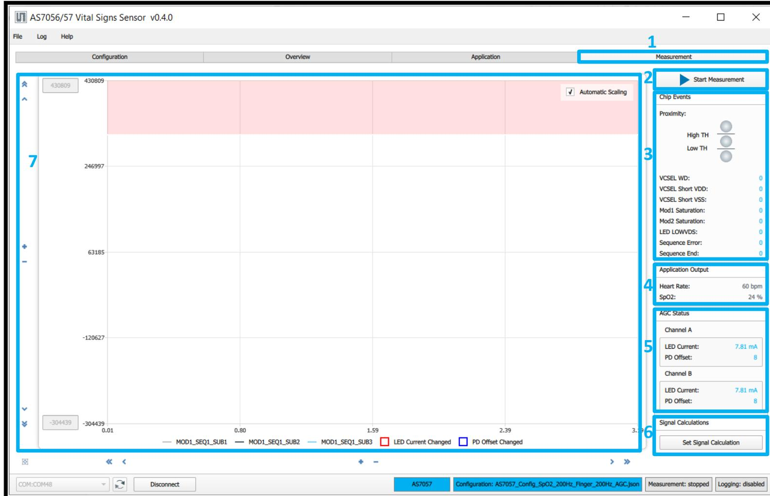
Fig. 10: Overview of SW GUI – Measurement Tab
