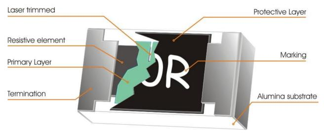
Fig 1. Construction of a Chip-R
