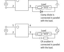
2) When Clamp diode or CR Snubber is used in the circuit, the spike voltages from the load are limited. But the longer wire may become the inductance and cause the spike voltage. Keep the wire as short as possible.
