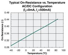
Typical On-Resistance vs. Temperature
