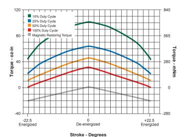
Graph 1 shows three position operation. In any mode, the armature seeks center of stroke at zero power.
