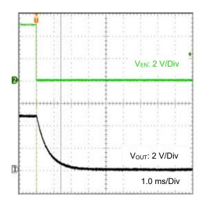
Figure 28. EN Shutdown Waveform (5 V output, I<sub>OUT</sub> = 1 mA)
