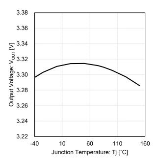
Figure 34. Output Voltage vs Junction Temperature (3.3 V output)
