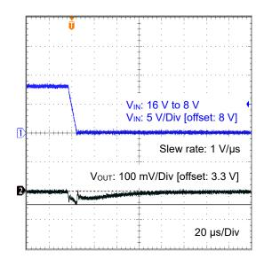
Figure 46. Line Transient 16 V to 8 V (3.3 V output, I<sub>OUT</sub> = 150 mA)
