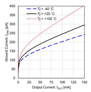
Figure 31. Ground Current vs Output Current (3.3 V output)
