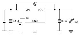
Measurement Setup for Figure 7, 35
