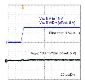
Figure 21. Line Transient 8 V to 16 V (5 V output, Iout = 0 mA)
