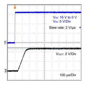
Figure 47. VIN Startup Waveform VIN: 0 V to 16 V (3.3 V output, I<sub>OUT</sub> = 0 mA)
