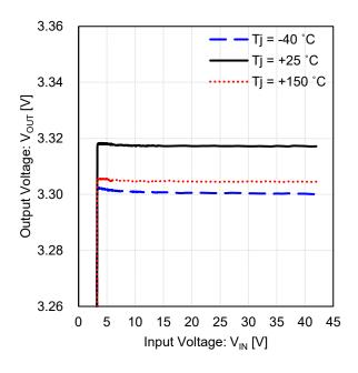
Figure 38. Output Voltage vs Input Voltage
