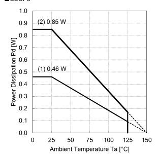
Figure 62. Power Dissipation Graph (SSOP5)
