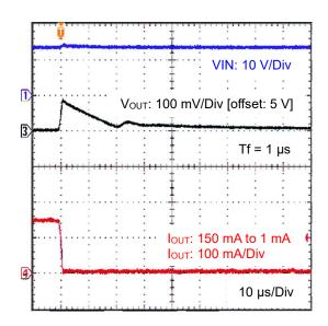
Figure 20. Load Transient 150 mA to 1 mA (5 V output, Tf = 1  $\mu$ s)
