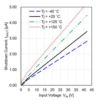
Figure 16. Shutdown Current vs Input Voltage (V<sub>EN</sub> = 0 V)
