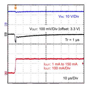
Figure 41. Load Transient 1 mA to 150 mA (3.3 V output, Tr = 1 µs)
