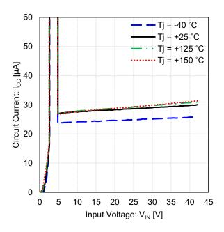
Figure 2. Circuit Current vs Input Voltage
