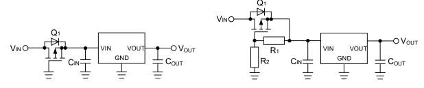
Figure 59. Protection against Reverse Polarity 2
