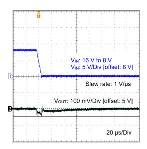
Figure 24. Line Transient 16 V to 8 V (5 V output, I<sub>OUT</sub> = 150 mA)
