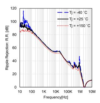
Figure 36. Ripple Rejection vs Frequency (3.3 V output, V<sub>Ripple</sub> = 1 Vrms, I<sub>OUT</sub> = 10 mA)
