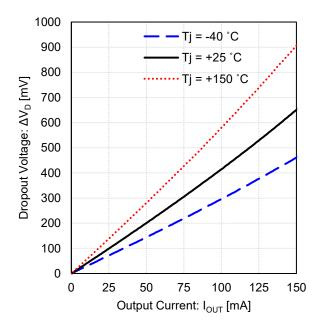
Figure 7. Dropout Voltage vs Output Current (5 V output, V<sub>IN</sub> = 4.75 V)
