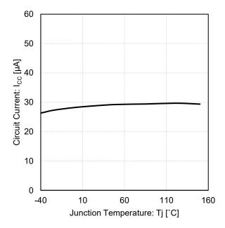
Figure 33. Circuit Current vs Junction Temperature (3.3 V output)
