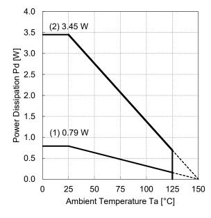
Figure 63. Power Dissipation Graph (HTSOP-J8)
