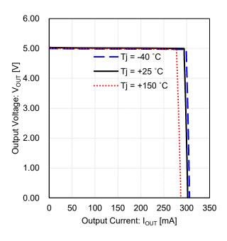
Figure 13. Output Voltage vs Output Current (5 V output, Over Current Protection)
