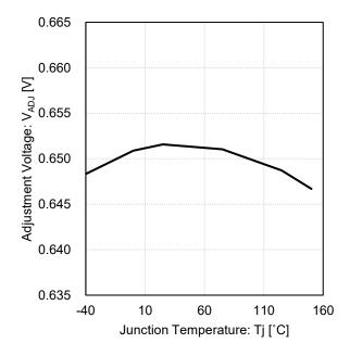
Figure 15. Adjustment Voltage vs Junction Temperature
