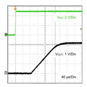
Figure 49. EN Startup Waveform (3.3 V output, I<sub>OUT</sub> = 1 mA)
