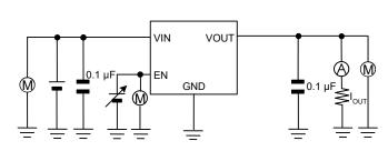
Measurement Setup for Figure 27 to 28, 49 to 50
