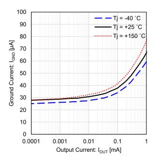
Figure 4. Ground Current vs Output Current \*magnification of Figure 3 at low output current (5 V output)
