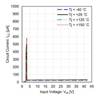
Figure 29. Circuit Current vs Input Voltage (3.3 V output)
