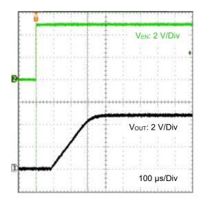
Figure 27. EN Startup Waveform (5 V output, I<sub>OUT</sub> = 1 mA)
