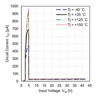
Figure 1. Circuit Current vs Input Voltage (5 V output)
