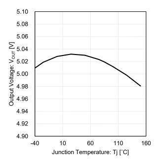
Figure 6. Output Voltage vs Junction Temperature (5 V output)
