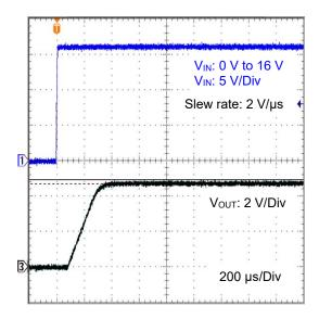
Figure 25. VIN Startup Waveform VIN: 0 V to 16 V (5 V output, I<sub>OUT</sub> = 0 mA)
