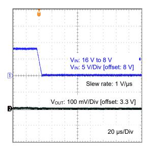
Figure 44. Line Transient 16 V to 8 V (3.3 V output, I<sub>OUT</sub> = 0 mA)
