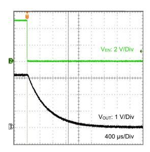
Figure 50. EN Shutdown Waveform (3.3 V output, I<sub>OUT</sub> = 1 mA)
