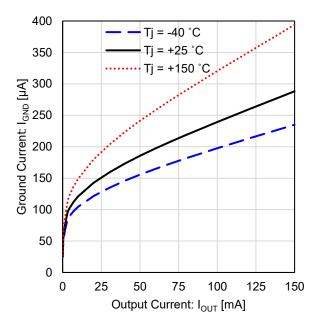
Figure 3. Ground Current vs Output Current (5 V output)
