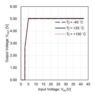
Figure 9. Output Voltage vs Input Voltage (5 V output)
