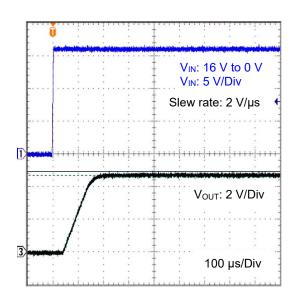
Figure 48. VIN Startup Waveform VIN: 0 V to 16 V (3.3 V output, I<sub>OUT</sub> = 150 mA)
