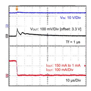
Figure 42. Load Transient 150 mA to 1 mA  $(3.3 \text{ V output, Tf} = 1 \mu\text{s})$
