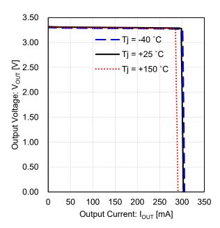
Figure 40. Output Current vs Output Voltage (3.3 V output, Over Current Protection)
