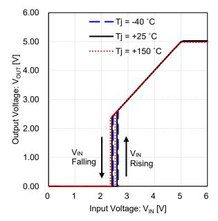
Figure 11. Output Voltage vs Input Voltage \*magnification of Figure 9 at low input voltage (5 V output)
