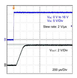
Figure 26. VIN Startup Waveform VIN: 0 V to 16 V (5 V output, I<sub>OUT</sub> = 150 mA)
