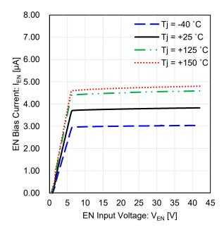
Figure 17. EN Bias Current vs EN Input Voltage
