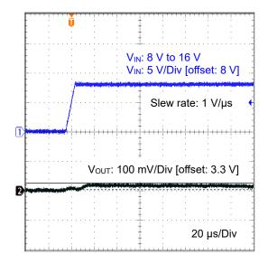
Figure 43. Line Transient 8 V to 16 V (3.3 V output, I<sub>OUT</sub> = 0 mA)
