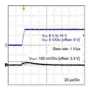
Figure 45. Line Transient 8 V to 16 V (3.3 V output, I<sub>OUT</sub> = 150 mA)
