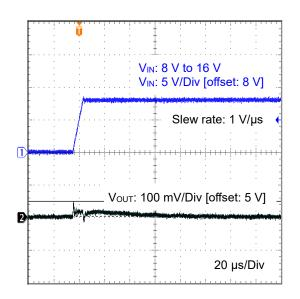
Figure 23. Line Transient 8 V to 16 V (5 V output, I<sub>OUT</sub> = 150 mA)
