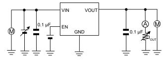
Measurement Setup for Figure 19 to 26, 41 to 48
