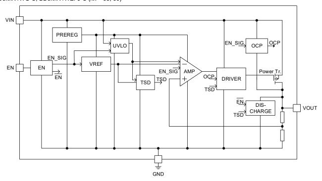
Applicable for product output voltage fixed type without Enable Function
