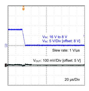
Figure 22. Line Transient 16 V to 8 V (5 V output, I<sub>OUT</sub> = 0 mA)
