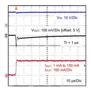
Figure 19. Load Transient 1 mA to 150 mA (5 V output,  $Tr = 1 \mu s$ )
