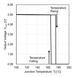
Figure 14. Output Voltage vs Junction Temperature (5 V output)
