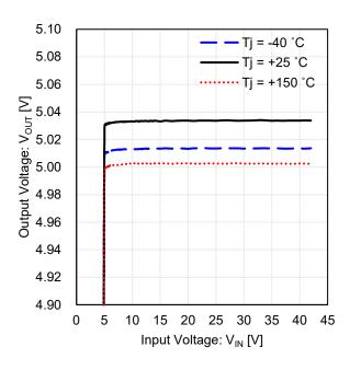
Figure 10. Output Voltage vs Input Voltage
