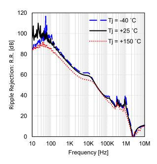
Figure 8. Ripple Rejection vs Frequency (5 V output, V<sub>Ripple</sub> = 1 Vrms, I<sub>OUT</sub> = 10 mA)
