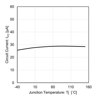
Figure 5. Circuit Current vs Junction Temperature (5 V output)
