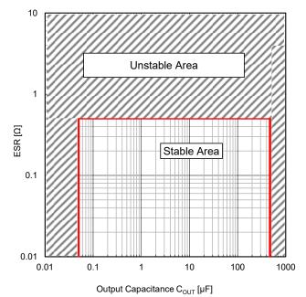
Figure 51. Output Capacitance C<sub>OUT</sub>, ESR Available Area (-40 °C  $\leq$  Tj  $\leq$  +150 °C, 4.5 V  $\leq$  V<sub>IN</sub>  $\leq$  42 V, V<sub>EN</sub> = 5 V, IOUT = 0 mA to 150 mA)
