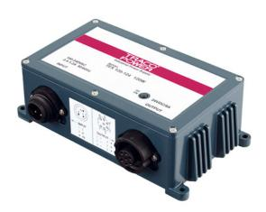
These power supplies have been designed particularly for applications in extreme environments. The rugged die-cast aluminium housing is water, ice, oil and dust resistant in compliance with IP67 and NEMA 4X standards. The metal case works as an efficient heatsink allowing full power operation at up to +60°C ambient temperature (no fan required). With a shock and vibration proof construction the power supplies can be mounted directly on a machine.
