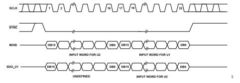
Figure 41. Daisy-Chain Diagram
