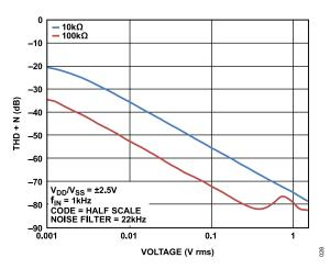
Figure 25. Total Harmonic Distortion Plus Noise (THD + N) vs. Amplitude
