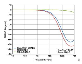
Figure 26. Normalized Phase Flatness vs. Frequency,  $R_{AB}$  = 100 k $\Omega$
