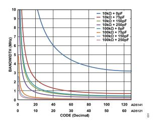
Figure 28. Maximum Bandwidth vs. Code vs. Net Capacitance
