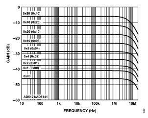
Figure 21. 10 kΩ Gain vs. Frequency vs. Code
