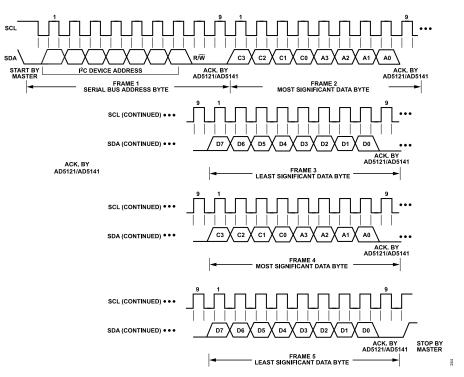
Figure 43. AD5121/AD5141 Interface Multiple Write
