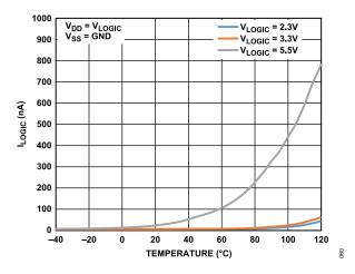
Figure 17. I<sub>LOGIC</sub> vs. Temperature
