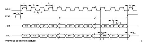
Figure 4. SPI Serial Interface Timing Diagram, CPOL = 0, CPHA = 1
