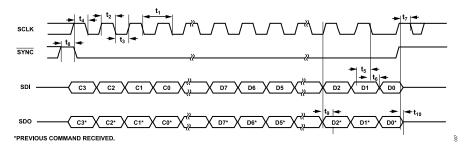
Figure 5. SPI Serial Interface Timing Diagram, CPOL = 1, CPHA = 0
