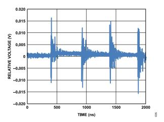
Figure 32. Digital Feedthrough
