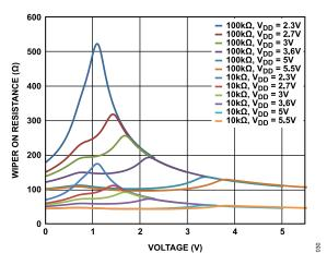
Figure 27. Incremental Wiper On Resistance vs. V<sub>DD</sub>
