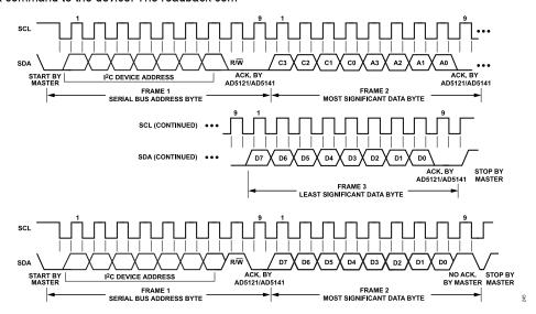
Figure 44. AD5121/AD5141 Interface Read Command
