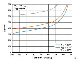
Figure 16. I<sub>DD</sub> vs. Temperature
