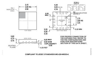
Figure 50. 16-Lead Lead Frame Chip Scale Package [LFCSP] 3 mm × 3 mm Body and 0.75 mm Package Height (CP-16-22)
