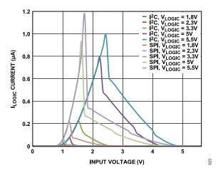
Figure 20. I<sub>LOGIC</sub> Current vs. Digital Input Voltage
