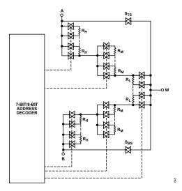
Figure 45. AD5121/AD5141 Simplified RDAC Circuit
