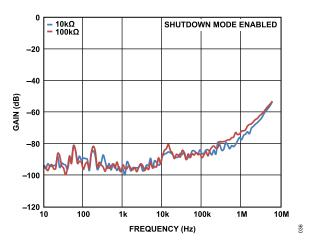
Figure 33. Shutdown Isolation vs. Frequency
