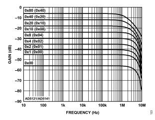
Figure 24. 100  $k\Omega$  Gain vs. Frequency vs. Code
