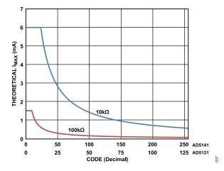
Figure 34. Theoretical Maximum Current vs. Code
