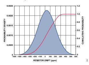
Figure 30. Resistor Lifetime Drift
