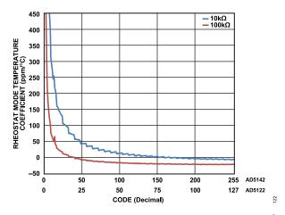
Figure 19. Rheostat Mode Temperature Coefficient ( $(\Delta R_{WB}/R_{WB})/\Delta T \times 10^6$ ) vs.
