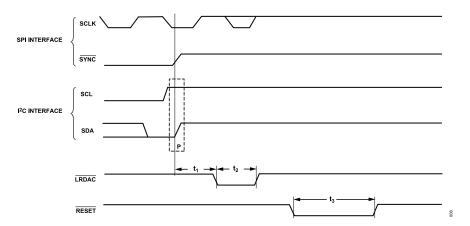
Figure 6. Control Pins Timing Diagram
