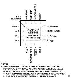
Figure 7. Pin Configuration
