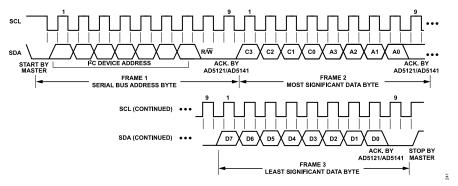
Figure 42. AD5121/AD5141 Interface Write Command
