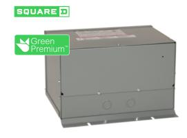
Low voltage transformer, encapsulated dry type, 3 phase, 3kVA, 480V primary, 208Y/120V secondary, Type 3R
