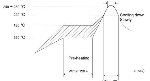
Please use the reflow within 2 times. Within 60 s Use rosin type flux or weakly active flux with a chlorine content of 0.2 wt % or less.
