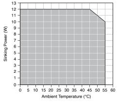
Figure 1. Sinking Power vs. Ambient Temperature Derating
