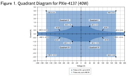
For additional information related to the Pulse Voltage or Pulse Current settings of the Output Function, for the PXIe-4137 (40W), including pulse on time and duty cycle limits for a particular operating point, refer to <u>Pulsed Operation</u>. For supplementary examples, refer to <u>Examples of Determining Extended Range Pulse</u> <u>Parameters and Optimizing Slew Rate using NI SourceAdapt</u>.
