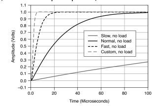
Figure 1.1 mA Range, No Load Step Response, Nominal
