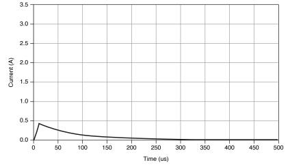
Figure 11. 10 µs Pulse Output with Load, Fast Transient Response
