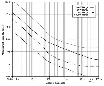
**Note** When the aperture time is set to 2 power-line cycles (PLCs), measurement noise differs slightly depending on whether the Power Line Frequency is set to 50 Hz or 60 Hz.
