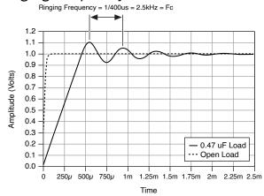
Compensation frequency and pole-zero ratio are used to determine the frequencies of the SMU control loop pole and zero, which can be used to optimize the system transient response by increasing phase margin and reducing ringing. To reduce the overshoot, it is recommended to set the compensation frequency close to the overshoot ringing frequency, see Fc in the figure above, and set the pole-zero ratio to be greater than 1.
