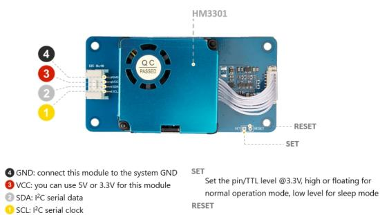
Module reset signal / TTL level @3.3V, low reset
