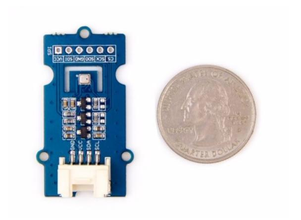
Grove - Temp&Humi&Barometer Sensor (BME280) is a breakout board for Bosch BMP280 high-precision, low-power combined humidity, pressure, and temperature sensor. This module can be used to measure temperature, atmospheric pressure and humidity accurately and fast. As the atmospheric pressure changes with altitude, it can also measure approximate **altitude** of a place. It can
