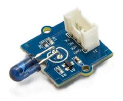
The Infrared Emitter is used to transmit infrared signals through an infrared LED, while there is an **Infrared receiver** to get the signals on the other side. An infrared LED is like any other LED, with its color centered around 940nm. We can not only use the emitter to transmit data or commands, but also to emulate remotes to control your home appliance using an Arduino. The Infrared Emitter can
