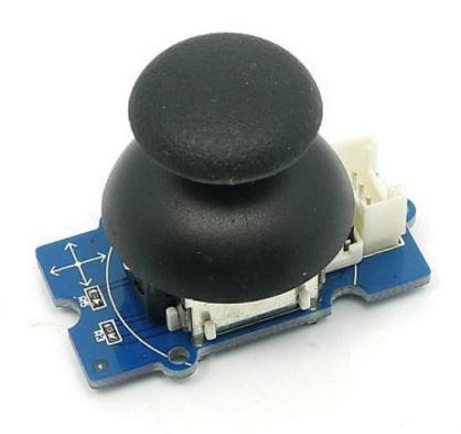
Grove - Thumb Joystick is a Grove compatible module which is very similar to the 'analog' joystick on PS2 (PlayStation 2) controllers. The X and Y axes are two ~10k potentiometers which control 2D movement by generating analog signals. The joystick also has a push button that could be used for special applications. When the module is in working mode, it will output two analog values,
