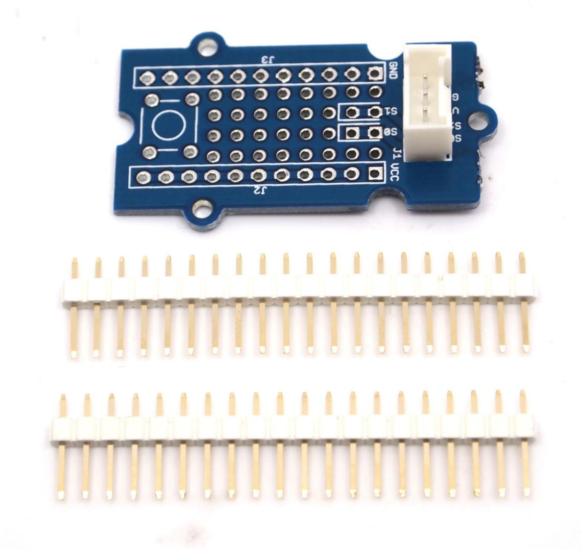
This Grove allows you to add your own circuitry or components to your Grove system prototypes. It gives you access to all four lines from the grove connector cable – S0, S1, VCC and GND. There is
