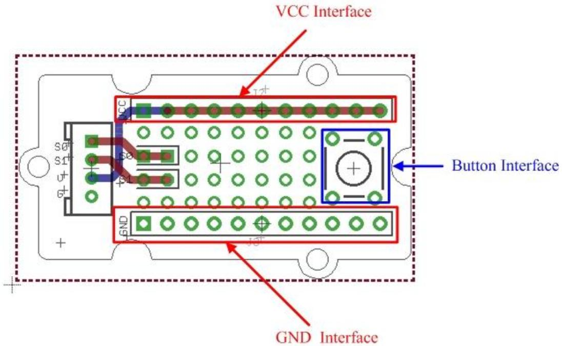
VCC and GND of the Grove interface are routed out as two buses as shown above. You can find soldering pads of Sig0 and Sig1 between two power buses.
