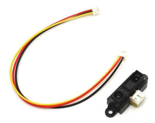
The 80cm Infrared Proximity Sensor is a General Purpose Type Distance Measuring Sensor. This sensor SharpGP2Y0A21YK, boasts a small package and very low current consumption, takes a continuous distance reading and returns a corresponding analog voltage with a range of 10cm (4") to 80cm (30"). Can be used in TVs, personal computers, cars and so on.
