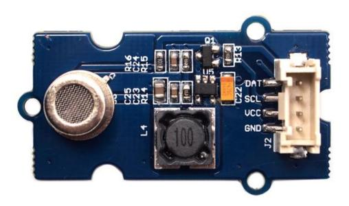
Grove - Alcohol Sensor is a complete alcohol sensor module for Arduino or Seeeduino. It is built with MQ303A
