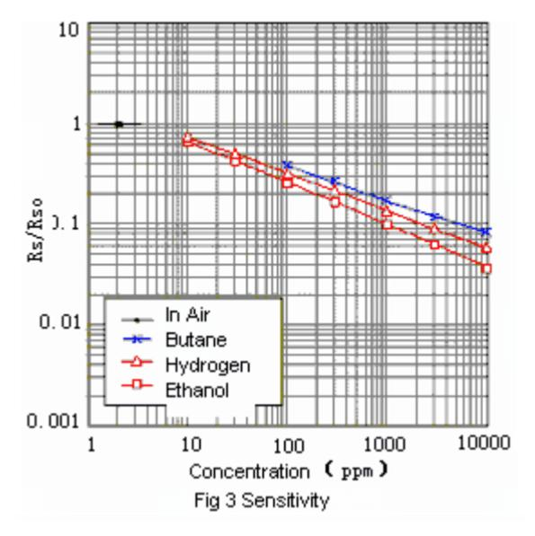
According to the figure, we can see that the minimum concentration we can test is 20ppm and the maximum is 10000ppm, in a other word, we can get a concentration of gas between 0.002% and 1%. However, we can't provide a formula because the relation between ratio and concentration is nonlinear.
