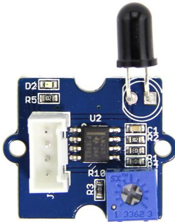
The Grove - Flame Sensor can be used to detect fire source or other light sources of the wavelength in the range of 760nm - 1100 nm. It is based on the YG1006 sensor which is a high speed and high sensitive NPN silicon phototransistor. Due to its black epoxy, the sensor is sensitive to infrared radiation. In fire fighting robot game,
