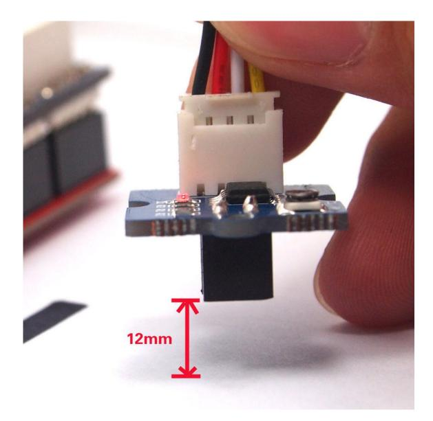
• **Step 4.** Adjust the potentiometer with a screwdriver to change the sensitivity of reflective photosensor, until the LED indicator glows. As your rotate clockwise, the reflective photosensor will be more sensitive to light.
