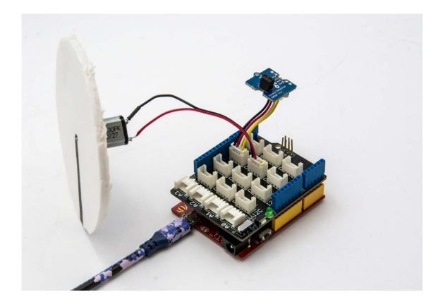
• **Step 3.** Attach a round, white paper plate (with a black line marked on it) to the motor. Place the sensor near this rotatory encoder. Run the motor.
