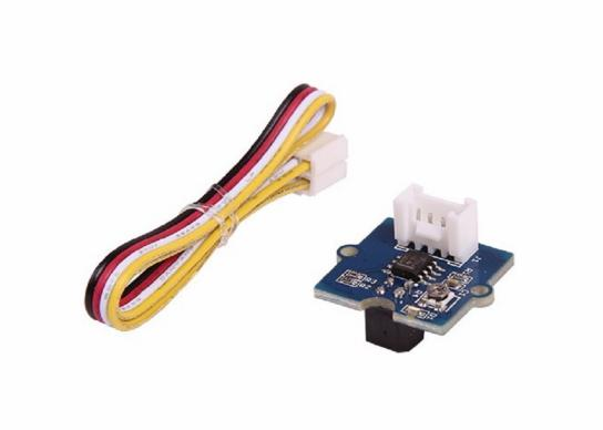
Grove - Infrared Reflective Sensor is used to detect the presence of an object within a specific range. The sensor consists of an IR LED and a photosensor (phototransistor) pair. The light emitted by the IR LED gets reflected by any object placed in front of the sensor and this reflection is detected by the photosensor(phototransistor). Any white (or lighter) colored surface reflects more than black (or darker) colored surface.
