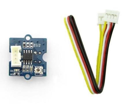
**Grove - IR Distance Interrupter** is used to detect any object blocking the path of light. The module consists of an IR LED and a photosensor (phototransistor) pair. The light emitted by the IR LED gets reflected by any object placed in front of the sensor and this reflection is detected by the photosensor(phototransistor). Any
