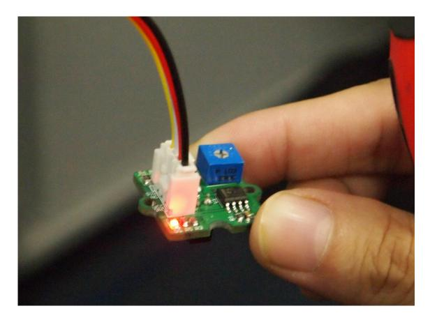
3.Adjust the potentiometer with a screwdriver to change the sensitivity of reflective photosensor, until the LED indicator glows. As your rotate clockwise, the reflective photosensor will be more sensitive to light.
