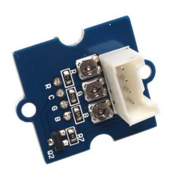
This Grove consists of one 8mm RGB LED. It operates at 5V DC. When SIG pin is logic HIGH, the RGB LED will light up. Perfect for use on Seeeduino digital outputs, or also can be controlled by pulse-width modulation. And it uses three adjustable resistor to change the color of the RGB LED.
