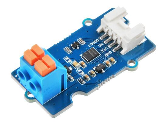
The Grove - 1-Wire Thermocouple Amplifier (MAX31850K) is a thermocouple-to-digital converters with 14-bit resolution and cold-junction compensation. This module is designed to be used in conjunction with a k-type thermocouple. The thermocouples have a much larger measurement range than thermistors. For example,
