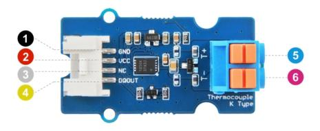
5 T+: Thermocouple Input, positive pole.
