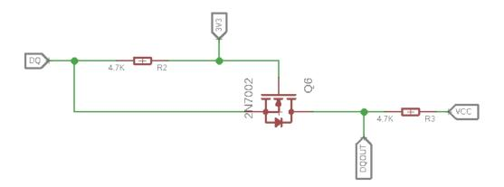
This is a typical Bi-directional level shifter circuit to connect two different voltage section. The left part, **DQ** pin of the MAX31850K use 3.3V, if the Arduino use 5V, this circuit will be needed. In the schematic above, **Q6** is N-Channel MOSFET 2N7002
