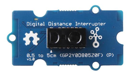
Grove - Digital Distance Interrupter 0.5 to 5cm is an infrared distance sensing module based on GP2Y0D805Z0F. Normaly the output of this sensor is 1(High), when the object enters the measurement range of the sensor, it will be triggered and output a
