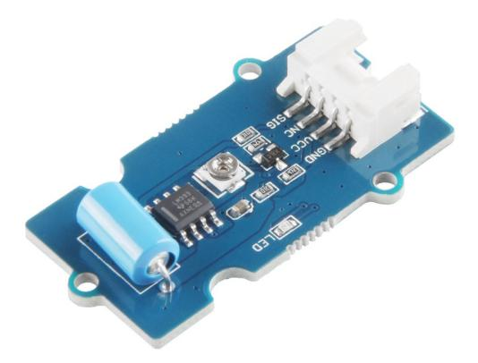
The Grove - Vibration Sensor (SW-420) is a high sensitivity nondirectional vibration sensor. When the module is stable, the circuit is turned on and the output is high. When the movement or vibration occurs, the circuit will be briefly disconnected and output low. At the same time, you can also adjust the sensitivity according to your own needs. All in all, this is a perfect module for vibration or tilt sensor.
