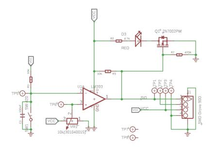
First, let's begin with the **SW1** which at the lower left corner. Actually, the **SW1** is the vibration module **SW-420**. When the module is in a stable state, the module is turned on. **Pin2** of **U1A** is connected to the **GND** though **SW1**.
